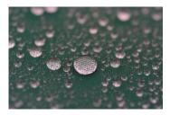
**Coating with Nanoparticles** On the shells of the Carbo-Drums with Carbo Look the surface is treated in a way that dirt hardly accumulates and is washed off whe...
